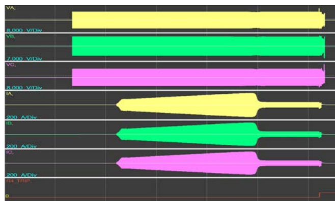
The Solcon Data Logger can diagnose an array of issues including a soft starter trip due to a network fluctuation (phase loss).
